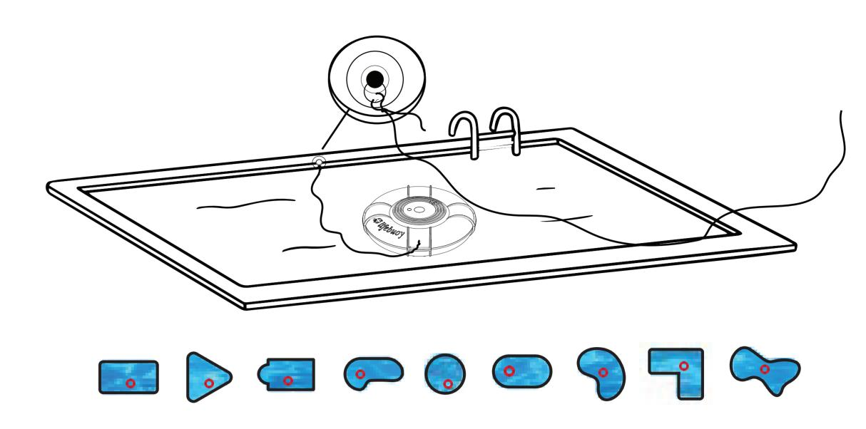
Install the home unit high up on a wall in dry place that is as close to the pool as possible.
